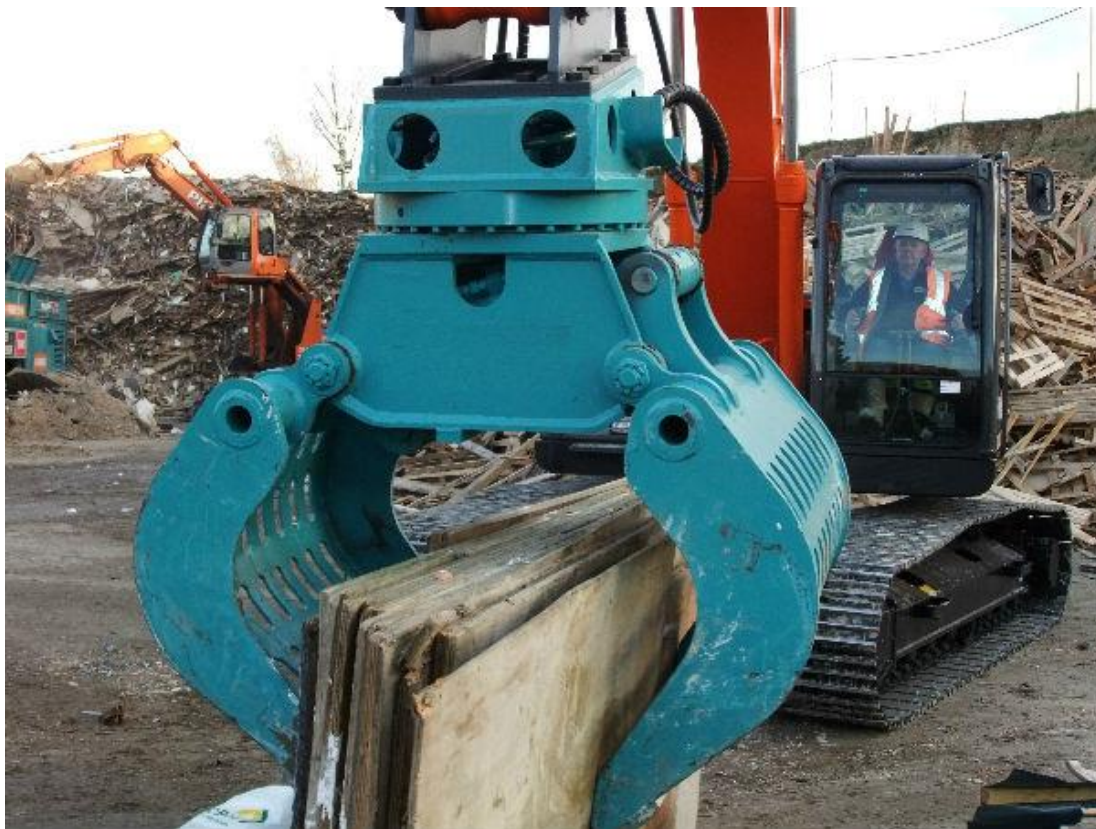
Figure 11: excavator with sorting grapple
