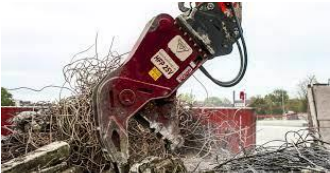
Figure 10: Excavator with fixed pulveriser
